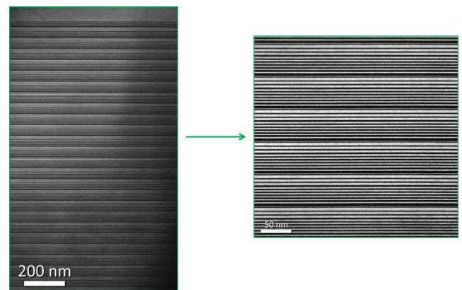
Figure 1 Transmission Electron Microscopy (TEM) of a QCL active region grown on the JR CCS Aixtron reactor
