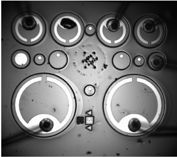
Figure 1. Photograph of the photodiodes showing the geometry of the top contacts. The photodiodes at the bottom of the figure are the 409 \mu\text{m} diameter devices; the photodiodes at the top are the 217 \mu\text{m} diameter devices.
